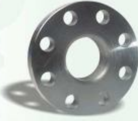
LAP - JOINT FLANGES 150 lb 1/2" a/to 24" -ANSI B 16-5-1977
